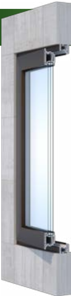
Exterior Glazed Window Vertical Cross Section
